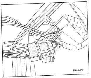
Plug connector -1- for the warning indicator switch back into the warning indicator switch.
