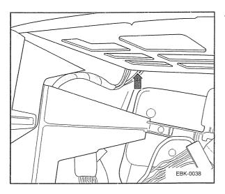
Now that the wiring is done, you can use a cable tie or other fastener to attach both the wiring and the convenience turn signal unit behind the built-in slot for the radio/navigation device.
