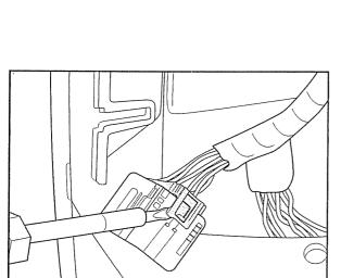
Insert Unlocking Tool VAS 3316 to unlock the radio navigation system, and then remove the radio/navigation system from the front.
