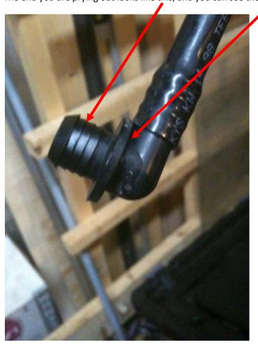
4. One you have the complete hose off the car; you want to remove the remaining nipple to make it flat/parallel to the hose. Reason being you are going to take a drill and drill the remaining nipple off and make the hole larger in the check valve.
