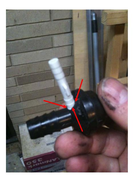
7. Insert the nipple in the pocket, I would advise <u>not</u> to put goop on the nipple before inserting it into the pocket, because the goop could ooze into the check valve and glue it shut/open.
