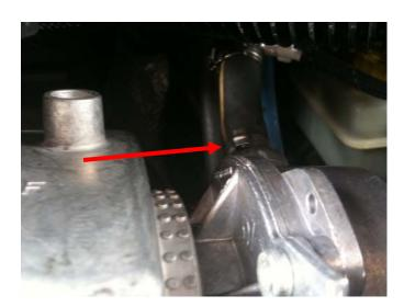
3. Now with a short flat head screw driver pry between the tube flange and the rubber on the brake booster end of the hose to pop it out of the brake booster. (CAUTION: Remember this hose is hard vinyl and can be easily broken) You don't have to pry hard, but in a couple places to pull it out of the rubber.
