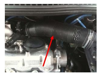
2. Carefully remove the pipe from the vacuum pump itself. (Depending on your situation, you may have to cut the rigid plastic pipe to get it off, or unclamp it, if it has been replaced before.)
