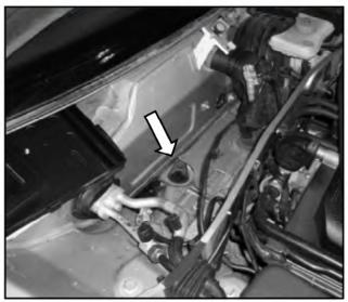
Section E – Clean Air Plenum Area and Remove Drain Tube
