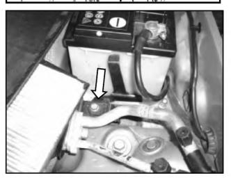
Remove bolt -arrow- and battery hold down bracket
