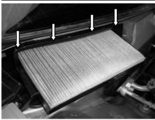
Reinstall plastic trough onto pollen filter housing - arrows -
