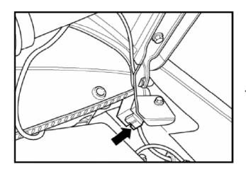
← Reinstall metal clip -arrow-on of cowl panel at driver side
