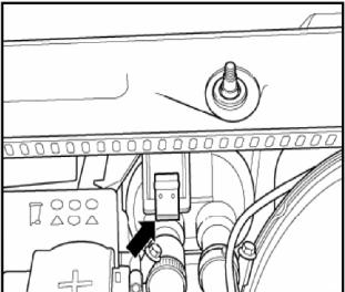
Remove metal clip-arrow- from center of cowl panel
