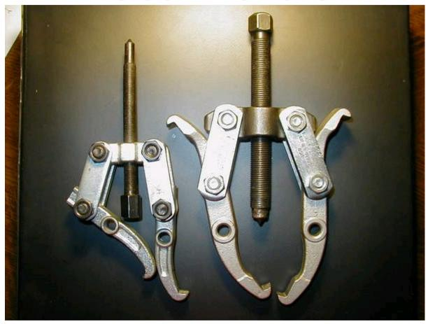
Compliments of velvetfoot these are the gear pullers I used. The big puller I used for the big gear. Some recommend griding down the very bottom of the finer so you can put it directly on the syncro gear. As this puller is currently, the part of the jaw just below the pulling surface is too thick to get between the syncro gear and the brass synchro on the 5<sup>th</sup> gear.
