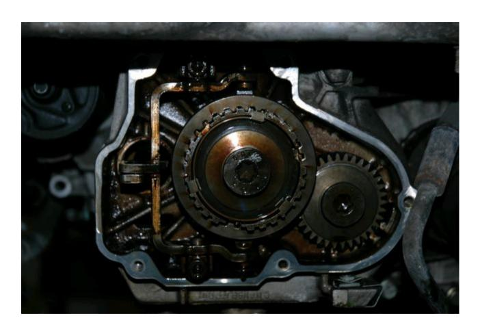
Remove the 2 bolts that hold the selector pivots into place. Once they are out the selector should easily fall right out. These should be the 3 square bolts.
