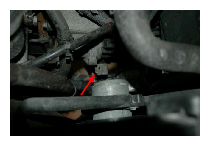
This is looking overhead into the engine bay. You want to remove the bolt that holds the power steering line here. This line kinda gets in the way of accessing the tranny.
