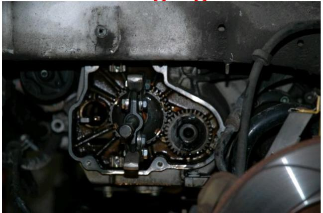
At this point you are ready to pull the gears off and you MUST do the big one first. On mine I tried heating the selector gear(not the the 5<sup>th</sup> gear you are replacing) and using the puller to pull on the 5<sup>th</sup> gear that I was actually trying to swap. This worked but required a lot of torque and I chipped a few teeth in the process but it did work. .... Please Read the next page for a possible alternative though.
