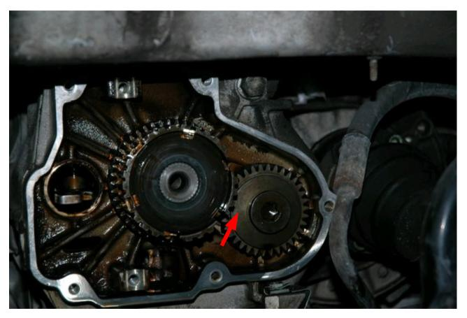
Both big bolts have a big washer behind them. Once you get them off you will want to take the washers off and then put the bolts back in. The gear puller needs something to push against and the bolt head works well. The bolts when it without the washer will allow you to pull the gear like 3/16 of an inch at which point you will need to remove the bolts to get the gear the rest of the way off.
