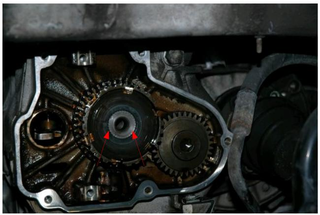
At this point you should check the position of the selector in relation to the shaft. You want to observe how flush it is with the end of the shaft so when you reinstall you have it just as far on as it was originally. You will also want to note the position of the small gear in relation to its shaft also.
