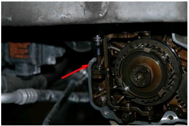
**This part is optional!** Once the end plate is off you will want to remove the small bolt that connects the selector to the selector shaft. This requires the T-45 Torx bit.
