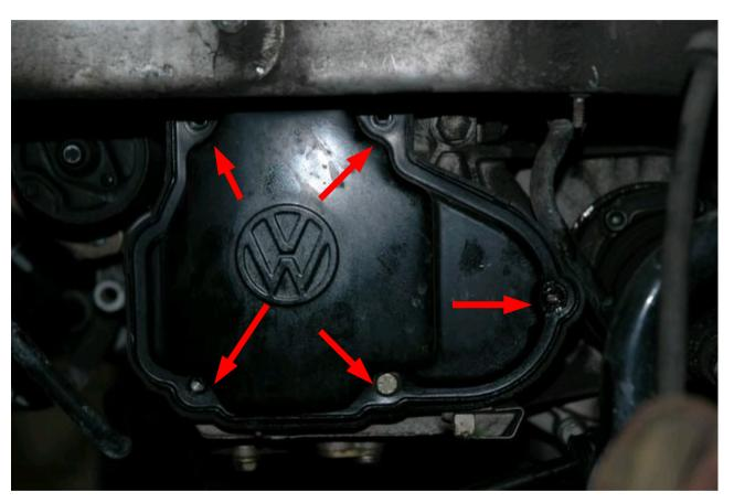
Next you want to remove the 5 bolts that hold the cover on to the end of the transmission. Remember when you get this cover off that some gear oil in the transmission will drain out so have someone nearby with a catch pan.
