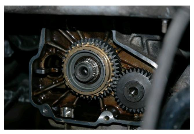
Put the synchro from the old gear on the new gear and swap the needle bearing over too then you can just slide it onto the shaft.
