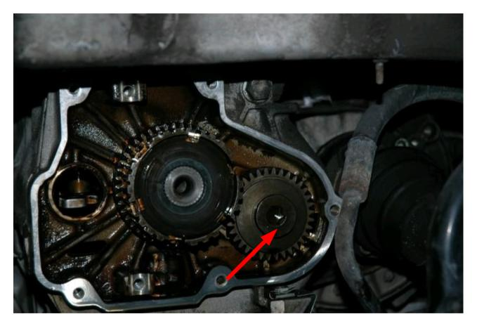
Next remove the 2 big 8mm 12 point bolts that hold on the little gear and the bigger selector gear. These will take some torque to come out and it may be helpful to have someone put the car in like 3<sup>rd</sup> gear and hold the brakes to keep everything from spinning as these take a good deal of torque. In the picture the bolt on the left gear is already removed.
