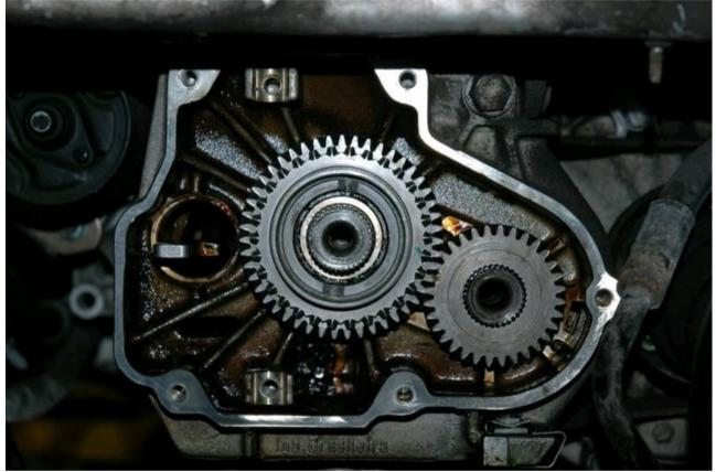
The new gears go on easy. Put the little gear on first. I started by carefully tapping the little gear on first with a rubber mallet until it wasn't going on easy any more. Once its that far on you can pull it down the rest of the way with the bolt and washer that hold it on. Too make this easier you should preheat these gears prior to installing.
