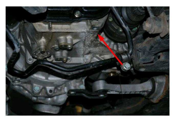
Then looking in from the wheel well you want to remove the bolt that holds the same line to the bottom of the transmission.
