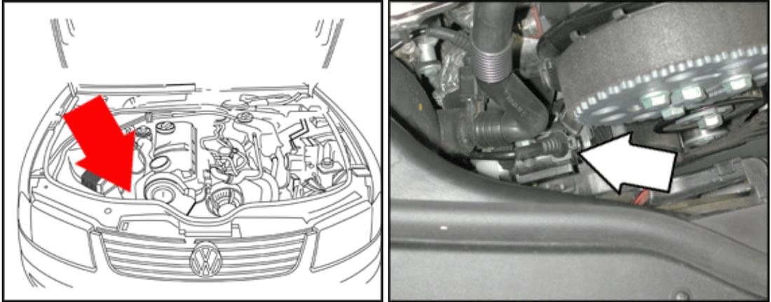
**N75 Wastegate Bypass Regulator Valve (2.0 ltr. tdi engine)**
