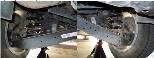
**2.** Support the wheel arm with a floor jack, slowly lower the floor jack and remove the lower transverse link (lower control arm) bolt and nut at the wheel bearing housing. **Take care! The wheel arm is under tension of the spring.** See fig 1
