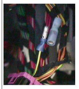
6. Now take out the fog relay and take the connector out of the panel the same way as drl relay connector. Find the gray/yellow wire on this connector. This should be pin 30 on the relay and pin 2 on the connector.
