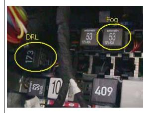
2. There are two nuts holding the relay panel in place. Take those two nuts off.
