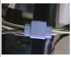
8. Attach a female connector at the other end of new wire and connect that to female connector you attached to the wires of the DRL relay.
