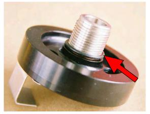
2. Using a little diesel fuel, lubricate the filter gasket and thread the fuel filter onto the filter adapter by hand. Once the filter is on the adapter hand tight tighten the filter one additional complete turn, using a pair of strap wrenches. It is helpful to put a mark on the filter to know when you have complete one full turn.
