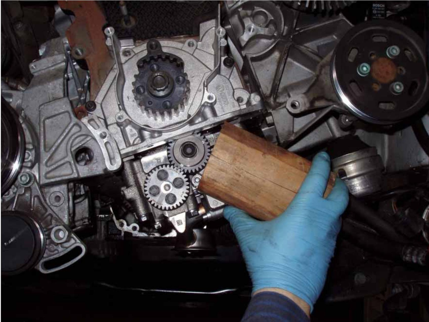
Tighten the intermediate gear bolt to 20 Nm plus ¼ turn with a 14mm XZN bit.
