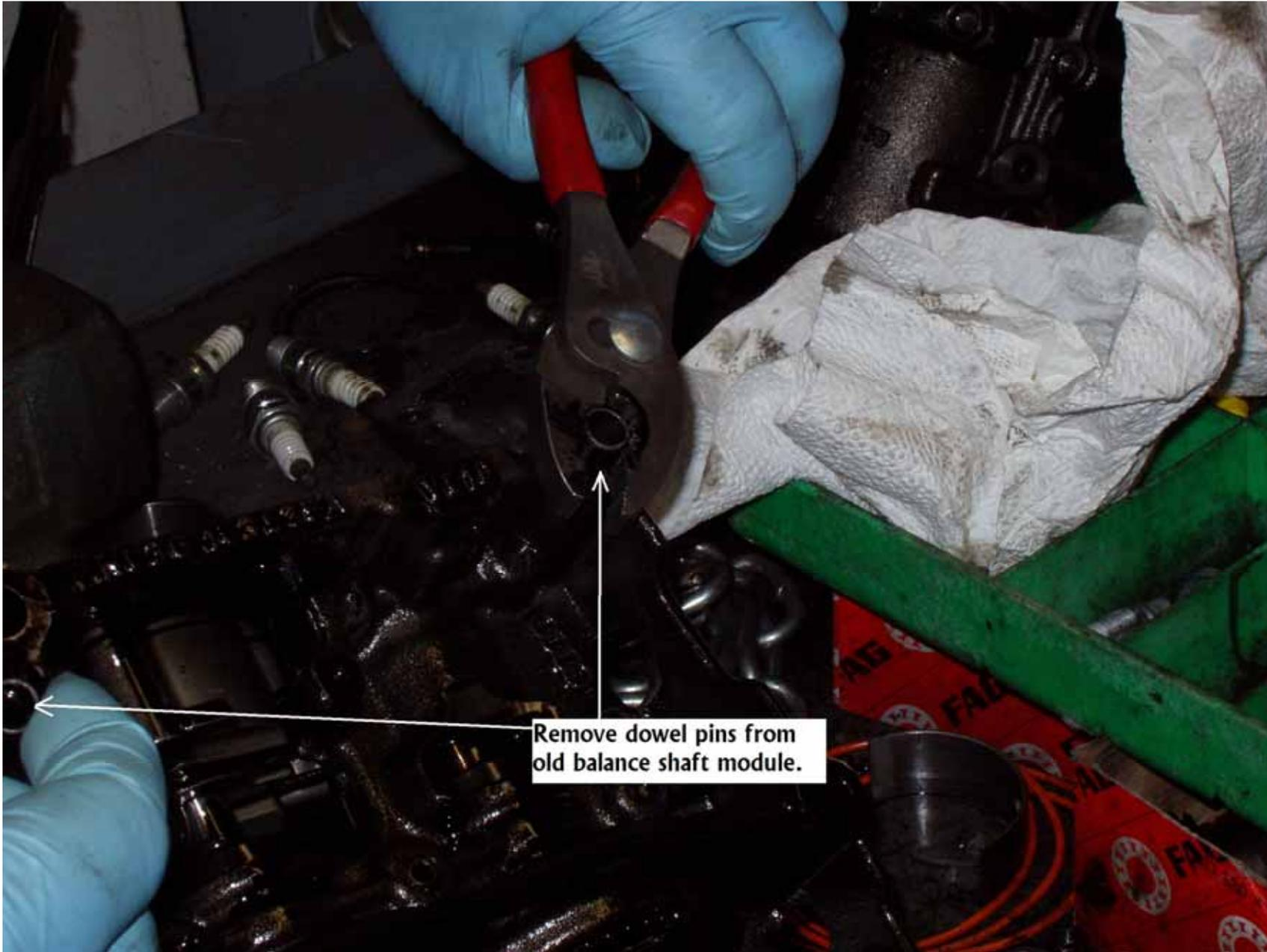
Remove dowel pins from old balance shaft module.
