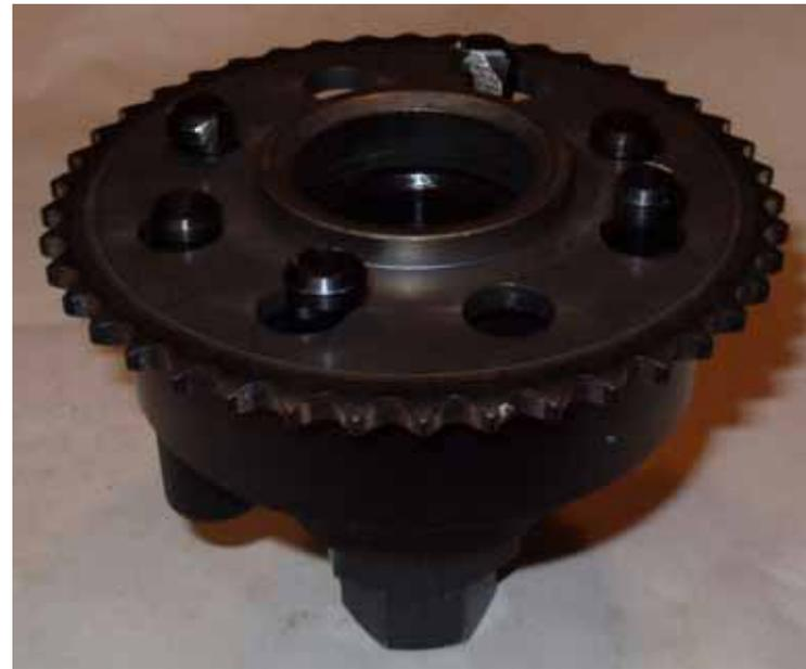
Counter hold the puller with a 32mm wrench (or an adjustable wrench), and use a 24mm socket or wrench to tighten the pressure screw. There will be a loud snap when the gear releases from the crankshaft. You will need to continue turning the pressure screw until the sprocket is complete free of the crankshaft.
