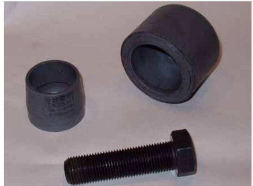
T10392 Puller – modify for 58mm spacing between pulling arms and round for the sprocket holes.
