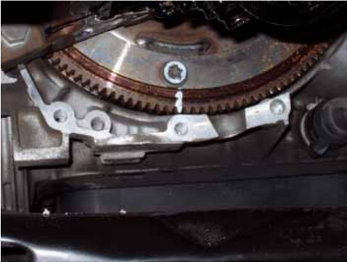
Remove the sealing flange from the front of the engine. Clean off old sealant from flange and engine block. Remove old crankshaft seal.
