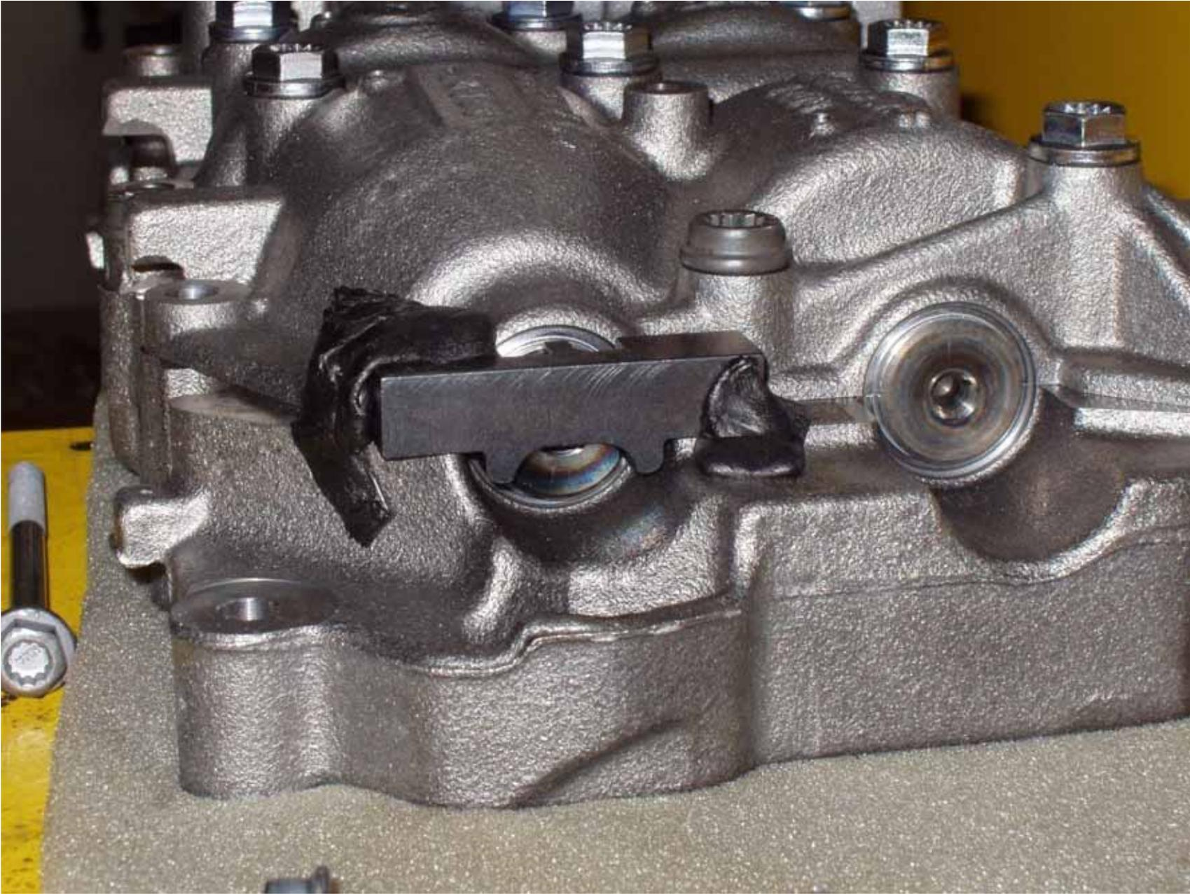
Install the previously removed dowel pins into the new balance shaft module.
