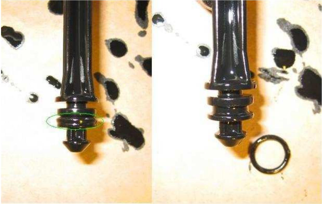
Remove the small O ring with the needle nose pliers. Notice where it is located, green circle.
