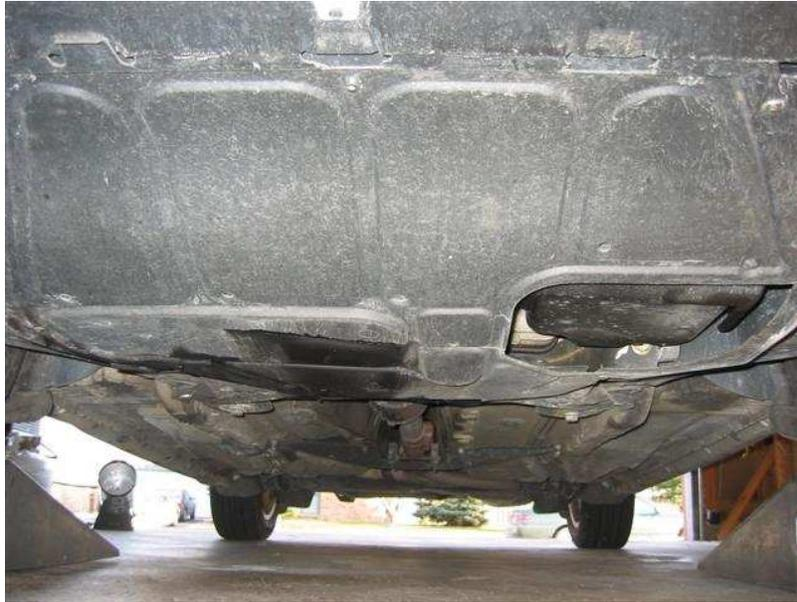
With the car on the ramps, crawl under or slide under if you have a creeper and remove all torx screws that are holding the belly pan. (Note: there is nothing wrong with my belly pan. It is all one perfect piece. I don't know why the picture appears to have part of it appearing to be ripped off. Honestly.)
