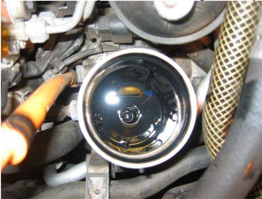
Notice the difference between the picture above and below. Use the baster to suck up the oil and dump it in the middle hole. It will drain to the pan. Oh yeah, there is plenty of oil there. There is a deep hole at the 6 o'clock position that you want to get it out. And a small hole in the 10 o'clock position.
