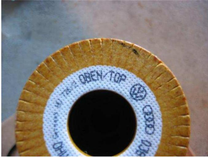
The filter has the word Oben/Top inked on it. (Oben is German for top.) That should be facing up in the housing. If you happen to not have any wording on it, then the two pictures below should help.
