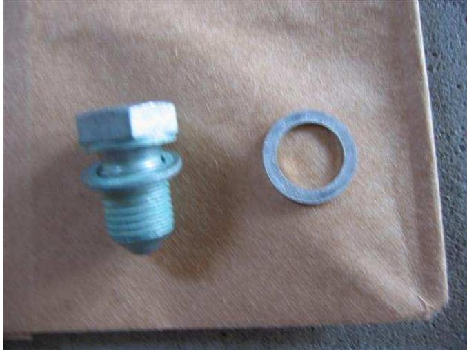
Check if you can easily removed the washer from the drain plug. If you can, then you may want to replace it with a crush washer. Lots of people re-use it. Newer cars, 2001+ have permanent washer. The part on the left in the picture above is the drain plug with permanent washer. It can't be remove, it can fool you thinking that it could but you can't easily. The part on the right in the picture above is a crush washer.
