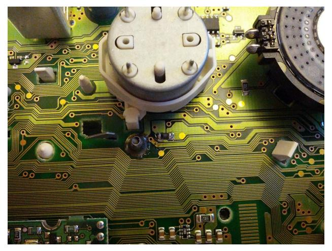
Turn the cluster back so the gauges are up. Now it's time to add the glow plug LED. The following photo shows the correct orientation of the LED. It will only work when installed in the correct direction. I didn't feel like removing all the white plastic framing but I was able to insert a small soldering iron straight down the hole and get it soldered into place.
