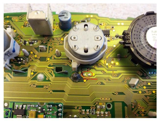
Here's a page that describes how to solder a surface mount resistor:
