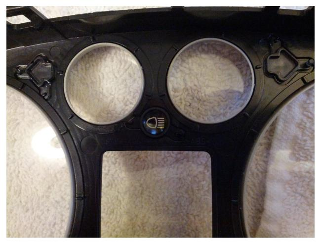
**Even though it looks like you can put the cluster back together now, don't do it yet.** You will need to flash the cluster with new software and then make sure the needles are lined up correctly by performing an output test with VCDS.
