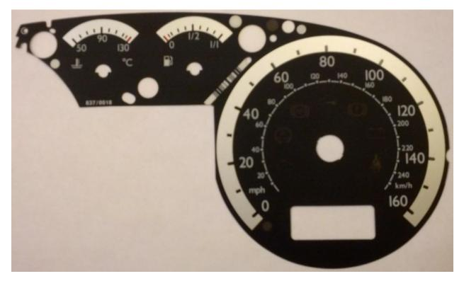
Place the faces on the cluster and screw the needles back in – again **counter**clockwise. Stop turning when they're simultaneously in the right position and the have the right gap between the face and needle. You should end up with something that looks like this:
