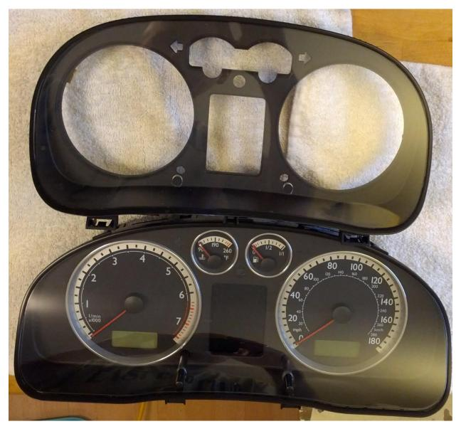
Since the tachometer red-line and speedometer don't match what's typically found in a TDI cluster, you'll need to replace the faces. You could probably use the faces from any Immo3 TDI cluster but the speedo will be wrong (top speed of 140mph vs. 160mph for the software you'll be flashing).
