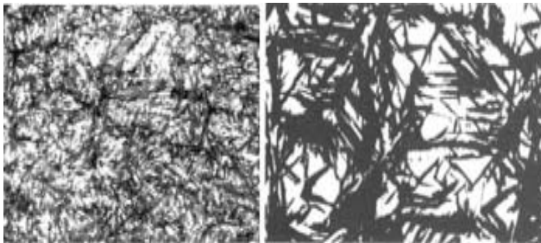
"Needle like" Structure of martensite
