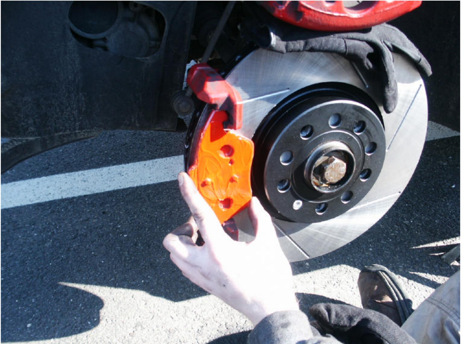
**Step 20:** Slide the caliper back onto the caliper carrier. Re-secure with the caliper carrier pins. Be sure to replace the black plastic covers on the caliper carrier pins, and reconnect the wear sensor if your new pads have one.
