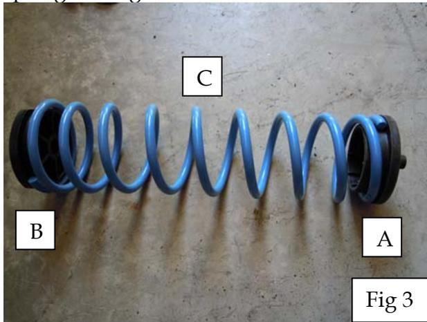
6. Turn the auxiliary spring **C** all the way into the main spring. Take care that the smallest diameter is mounted at the top. See Fig. 4
