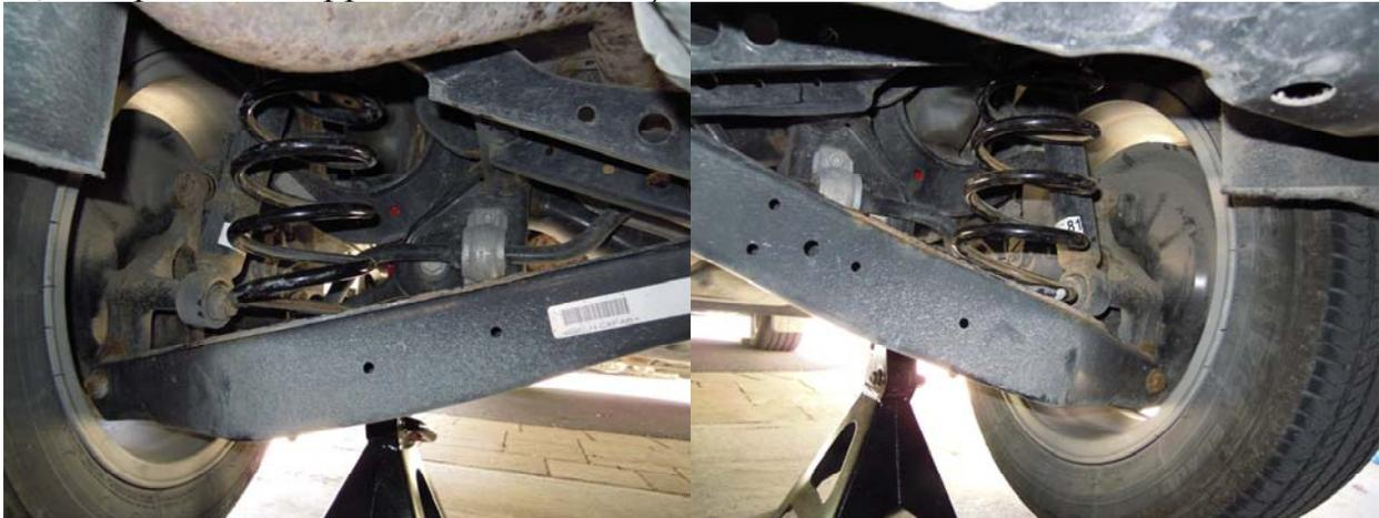
2. Support the wheel arm with a floor jack, slowly lower the floor jack and remove the lower transverse link (lower control arm) bolt and nut at the wheel bearing housing. **Take care! The wheel arm is under tension of the spring. See fig 1**
