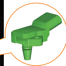
Charge Air Pressure Sensor G31 and Intake Air Temperature (IAT) Sensor G42
