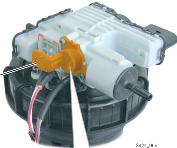
Reducing Agent Metering System Pressure Sensor G686
