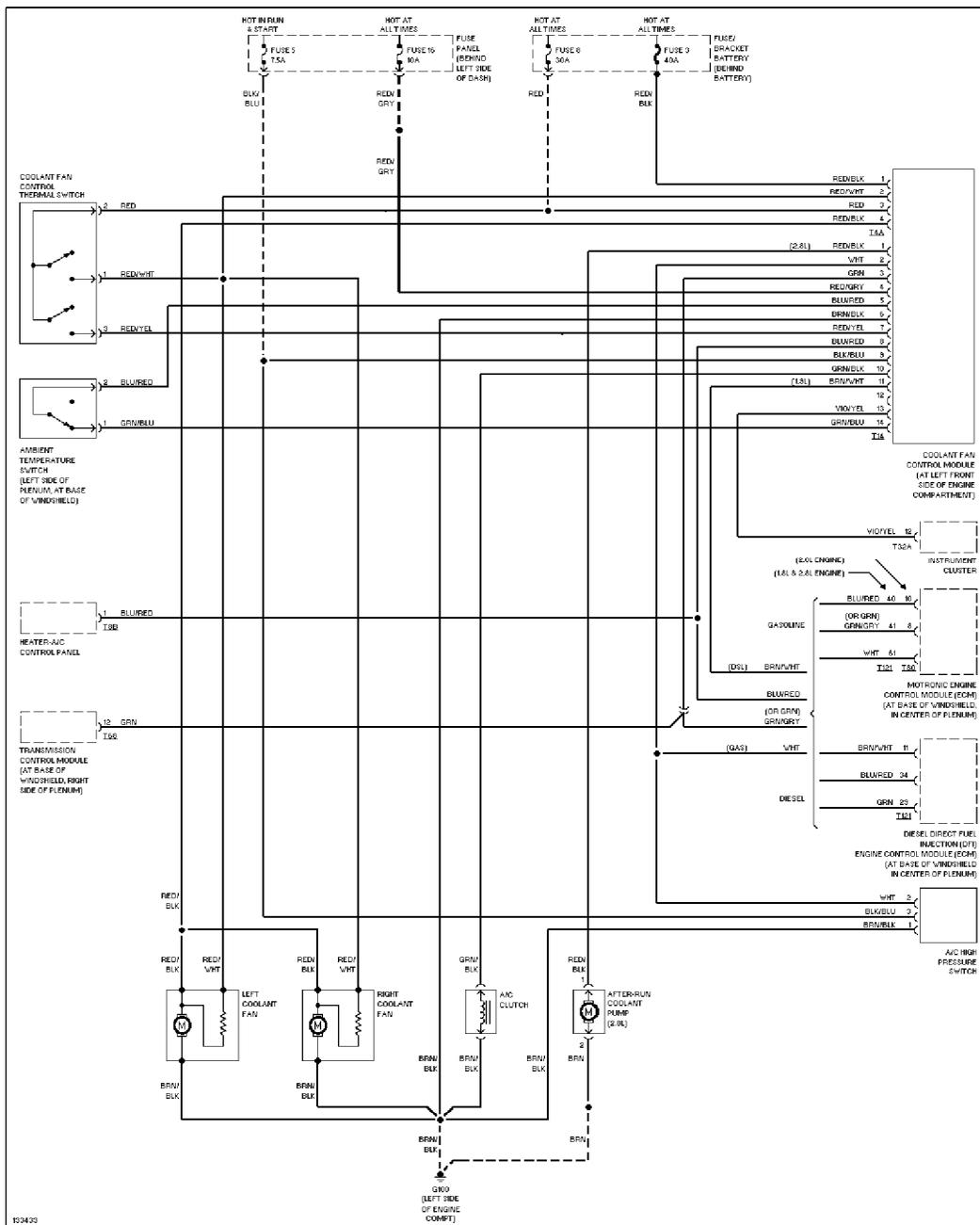
Cooling Fan Circuit, Manual A/C
