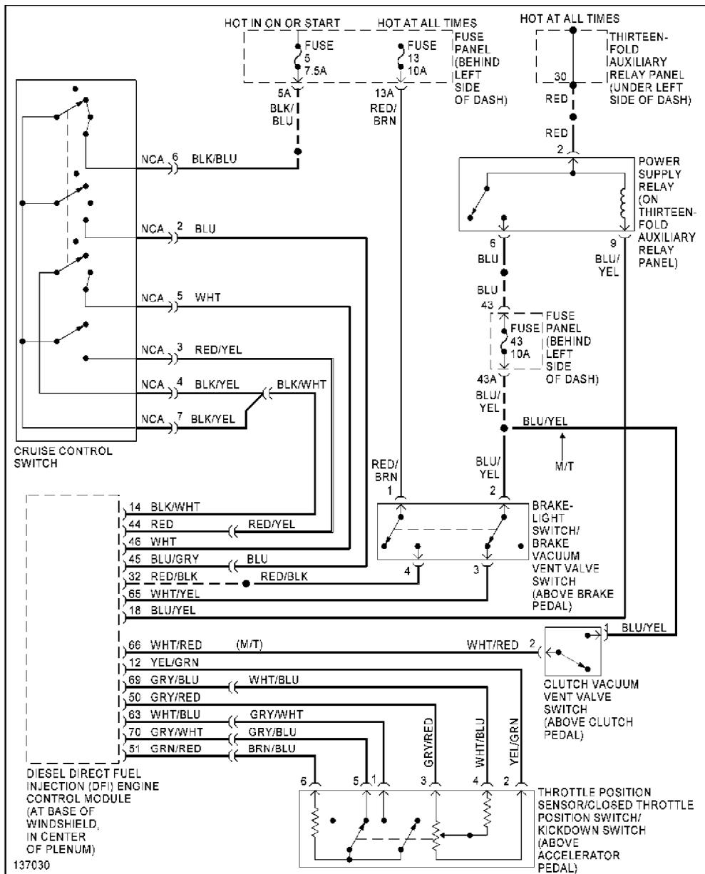
1.9L Turbo Diesel, Cruise Control Circuit
