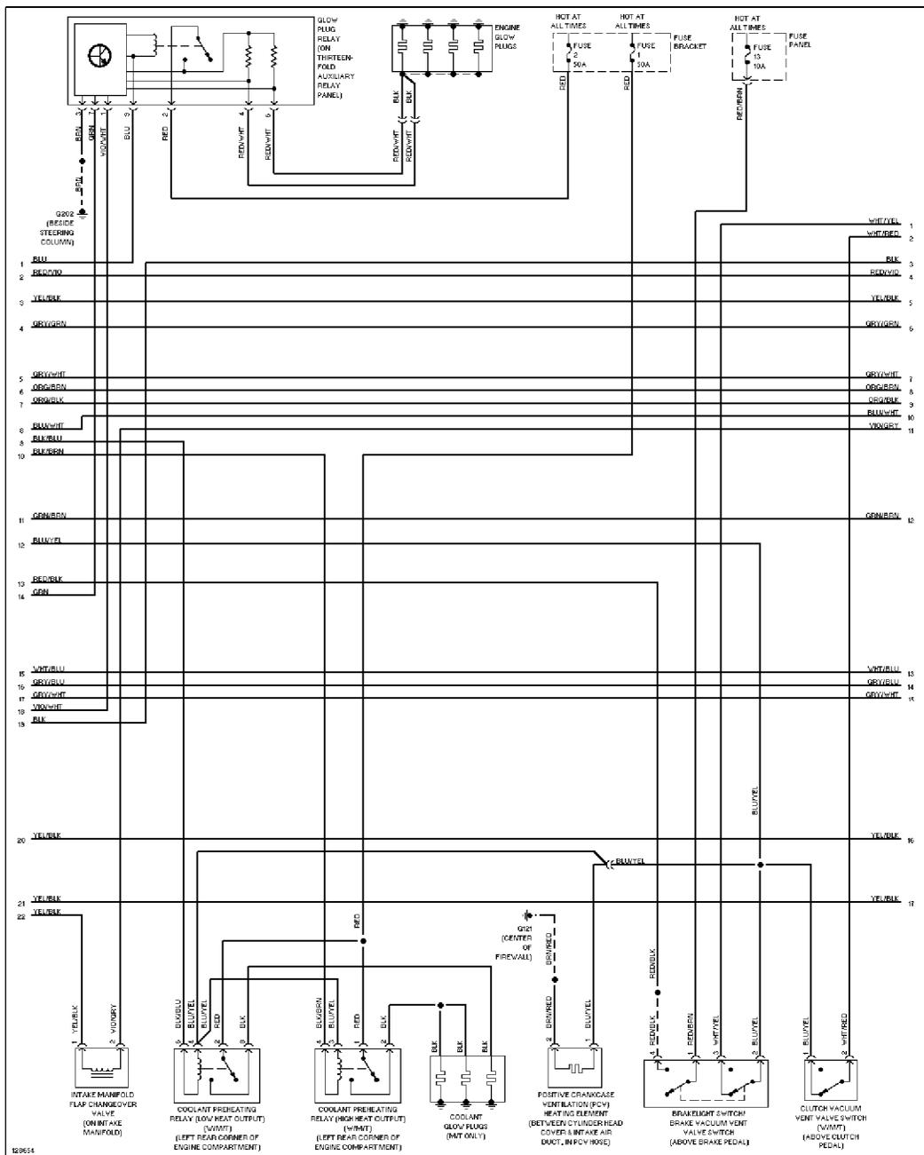
1.9L Turbo Diesel, Engine Performance Circuits (2 of 3)
