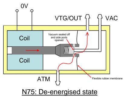
Note: if vacuum seal is leaking, then vacuum (VAC) can suck from atmosphere (ATM)
