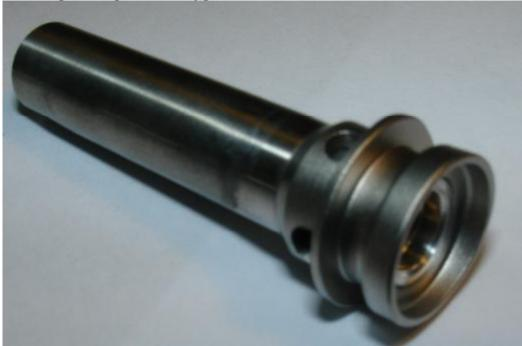
The part of the spool which gets dirty is inside here. The bottom of the hole is a seal which can move further inside. The area inside the 4 ports also gets dirty. The photo shows after I cleaned it. Sorry, I didn't think to take photos when it was dirty.
