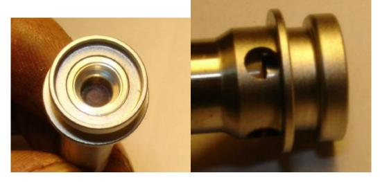
The valve head is shown next. The centre pipe is the vacuum line, which is connected to the bottom pipe connector (VAC). The other connection is OUT, connected to the VGT actuator. The end of the pipe normally seals against the seal shown at the bottom of the hole in the spool, in the de-energised state.
