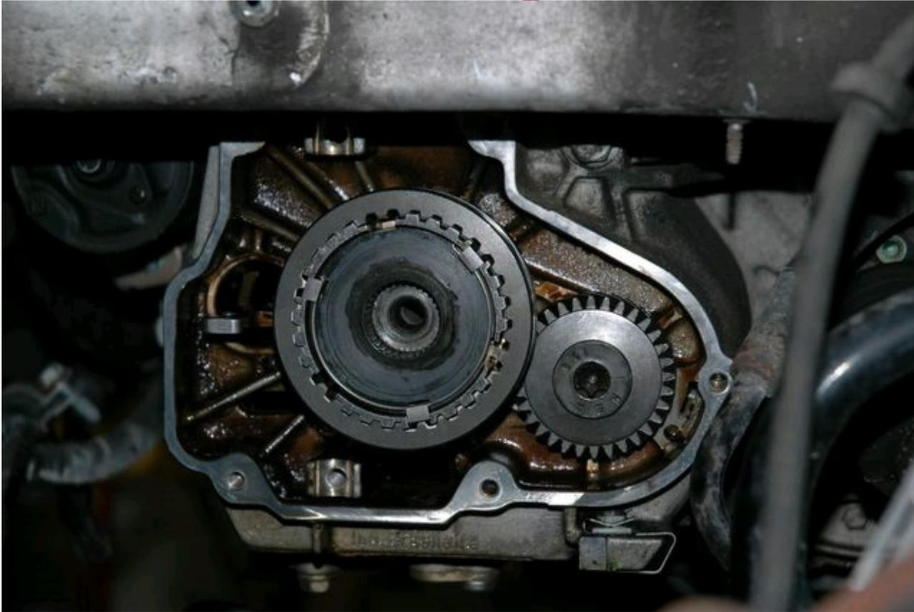
Once you have the selector assembly together its time to get it back on the shaft. Again I used the rubber mallet to get it started and then tightened it down using the washer and bolt that holds it on
