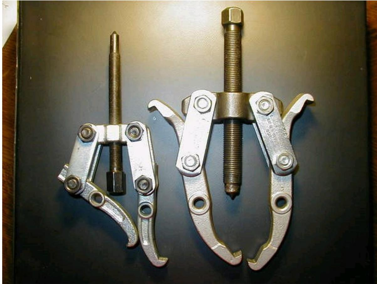
Compliments of velvetfoot these are the gear pullers I used. The big puller I used for the big gear. Some recommend grinding down the very bottom of the finer so you can put it directly on the syncro gear. As this puller is currently, the part of the jaw just below the pulling surface is too thick to get between the syncro gear and the brass synchro on the 5<sup>th</sup> gear.
