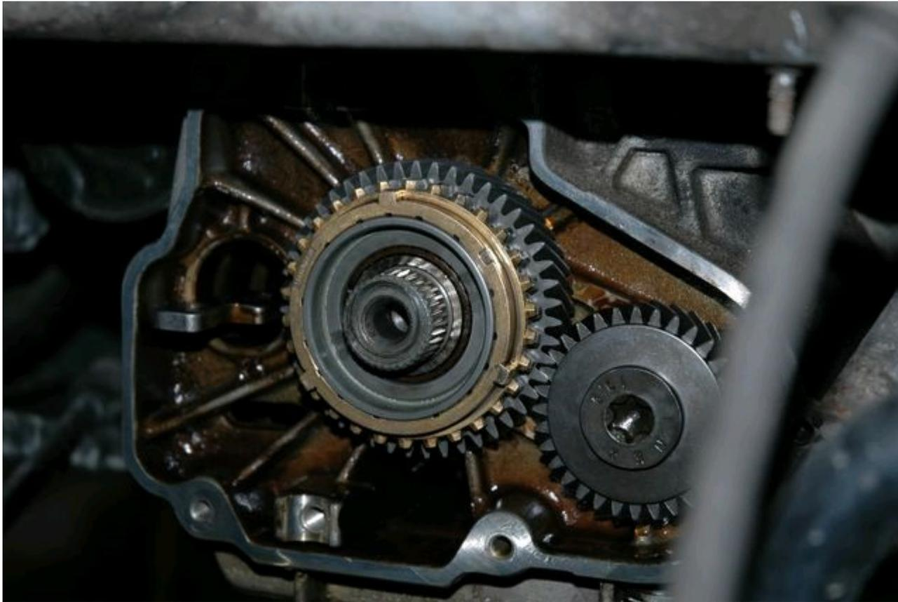
Put the synchro from the old gear on the new gear and swap the needle bearing over too then you can just slide it onto the shaft.
