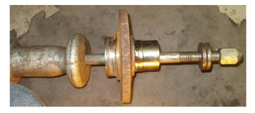
If the bearing race came out with the hub, you will need to use a bearing separator and appropriate other tools (e.g. press) to remove the race.
