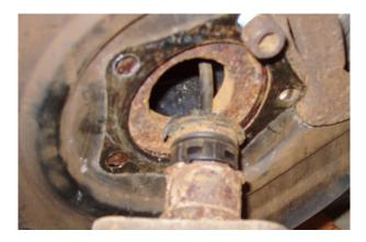
The alternative method is to use tool 80-200. After removing the clip and before unbolting the bearing, use this tool as a pry tool. It fits where the clip was and one can pry out the sensor provided it isn't really stuck hard into the bearing.
