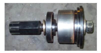
Counter hold the long nut with a 32mm box wrench or socket and wrench. Use an impact wrench such as the one mentioned above with an impact socket on the bolt to tighten the bolt and thus extract the bearing. Mine was 27mm but the kits have been known to vary.
