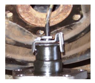
Lightly grease the sensor around the o-ring seal on it with a thin coating of wheel bearing grease.
