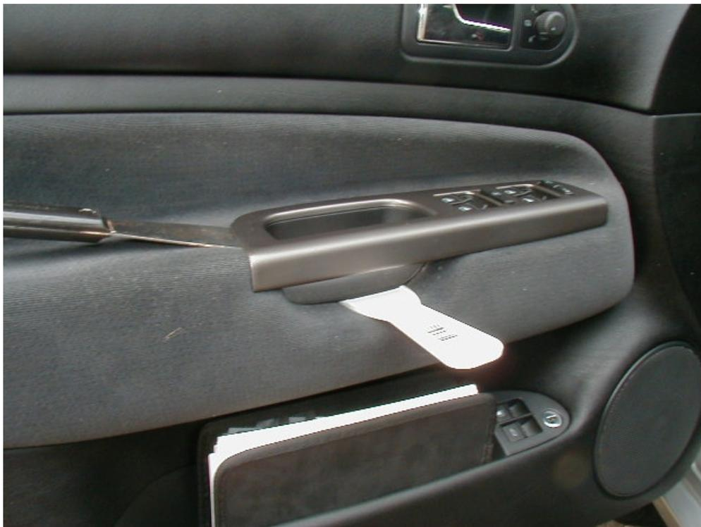
Pry up. You can use another knife underneath the handle part to assist in removing
