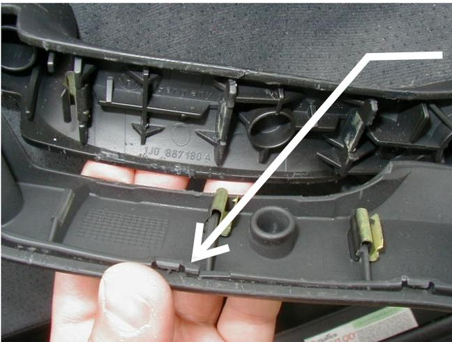
(4) tabs on the outer part help hold the handle together
