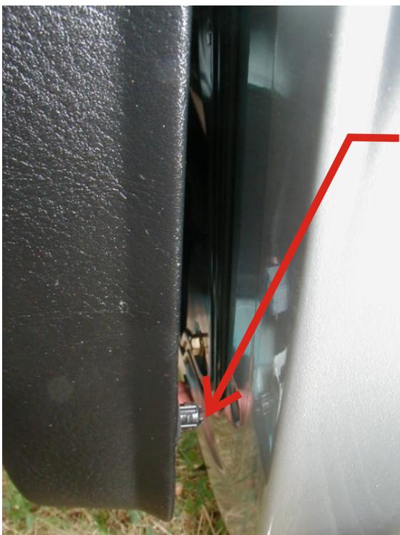
Start at the bottom using a stiff putty knife. Locate each clip and pry slowly until it releases
