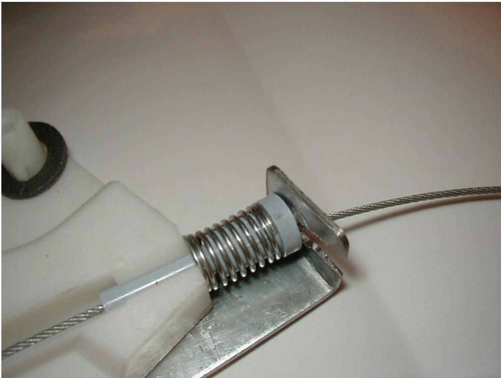
Keeps spring tension on both cables and maintains proper alignment to cables
