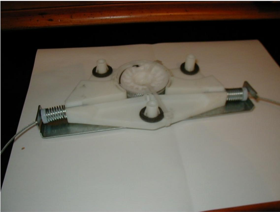
New cable guide with repair kit
