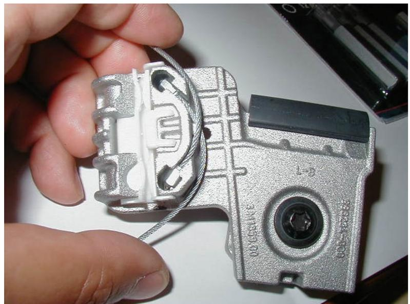
Remove one corner cable from the pulley. This slack will allow you to attach each cable end to the new clip
